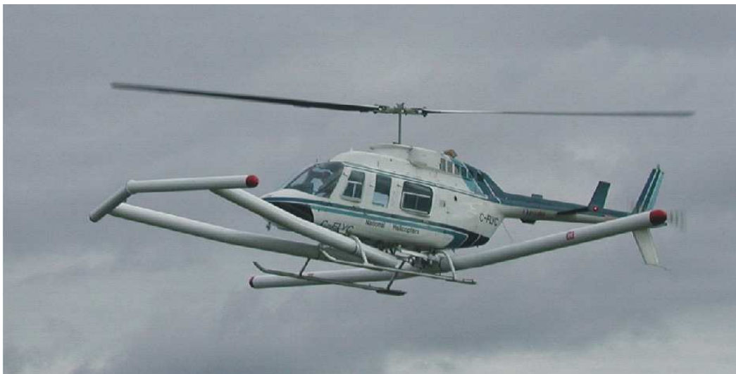
Figure 2.2 ORAGS-Arrowhead helicopter total field magnetometry system.
