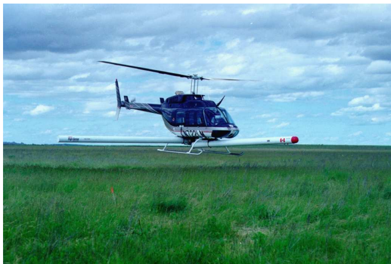
Figure 2.3 The HM-3 helicopter magnetometry system used by ORNL in 1999 for surveys at Badlands Bombing Range.
