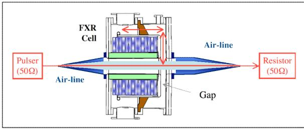
**Figure 1.** A cross section of the cell interior and air-line shows the power flow from the pulsar and reflections.
