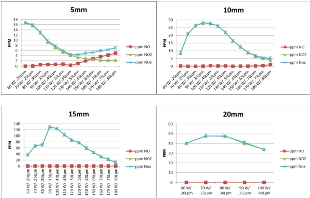
Figure 4. ppm at varying distances of Surfex® – Atomflo™ AH-250C - Testo-350 Diagnostics, Acquisition Software and Plasma Data Comparison
