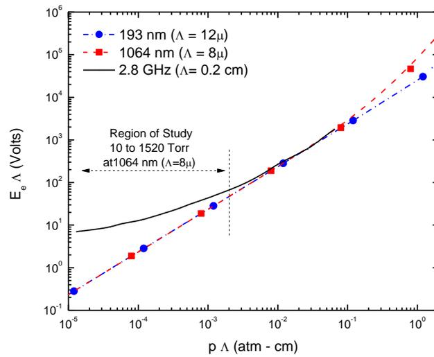
FIG. 1. Universal plot of microwave breakdown theory at 2.8 GHz with  $\Lambda = 0.2$  cm (solid line) extended to laser breakdown at  $\lambda = 1064$  nm with  $\Lambda = 8$  microns (square, dash) and  $\lambda = 193$  nm with  $\Lambda = 12$  microns (circles, dash-dot-dash).
