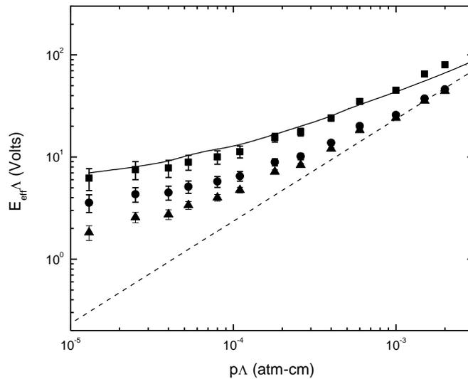
FIG. 6. Universal plot of (triangles) experimental 1064-nm laser breakdown threshold fields in dry air (with 0.1- $\mu\text{m}$  filter) compared with (solid line) microwave theory. (Dotted line) Microwave theory extended to  $\lambda = 1064$  nm. (Circles) MPI-corrected breakdown threshold data. (Squares) Data in circles scaled by a factor of 1.74.
