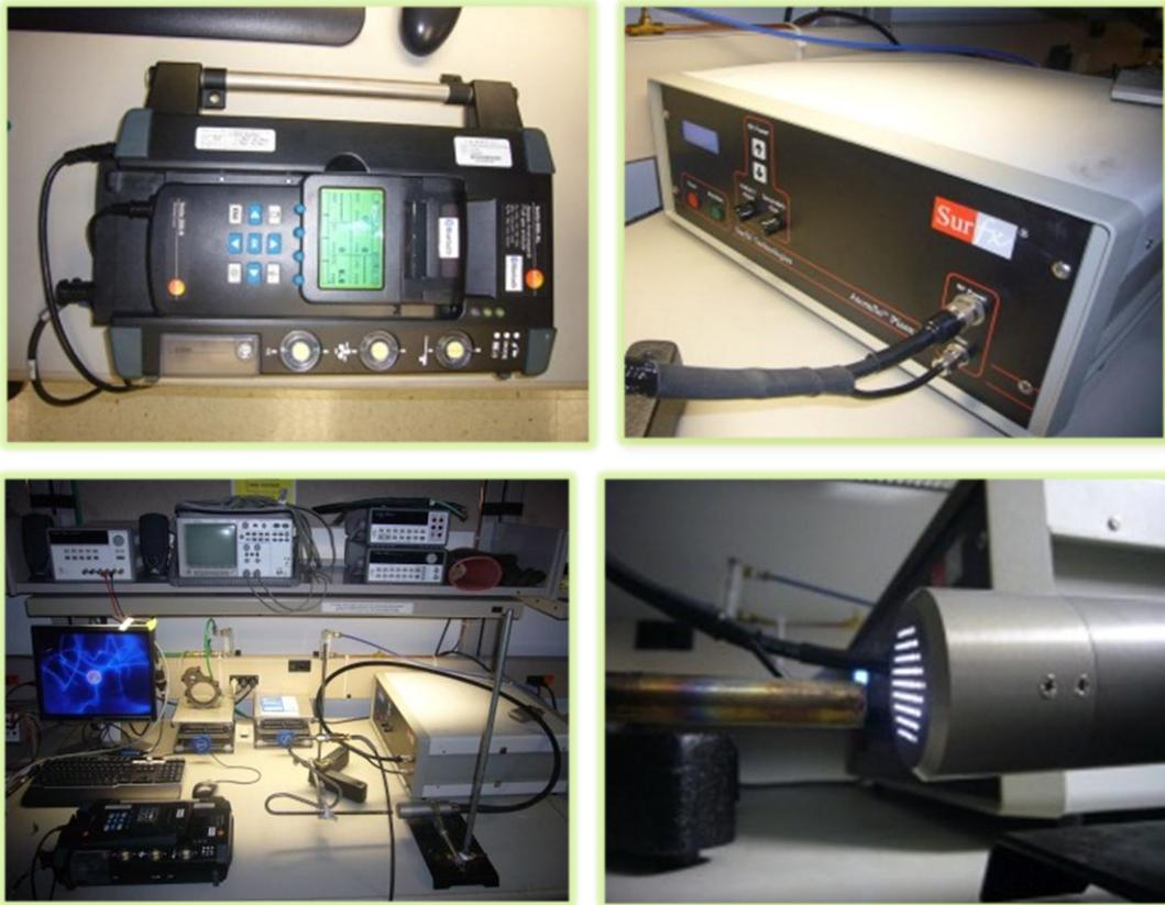
**Figure 3. Setup a 13.56 MHz radio frequency dielectric barrier plasma system**
