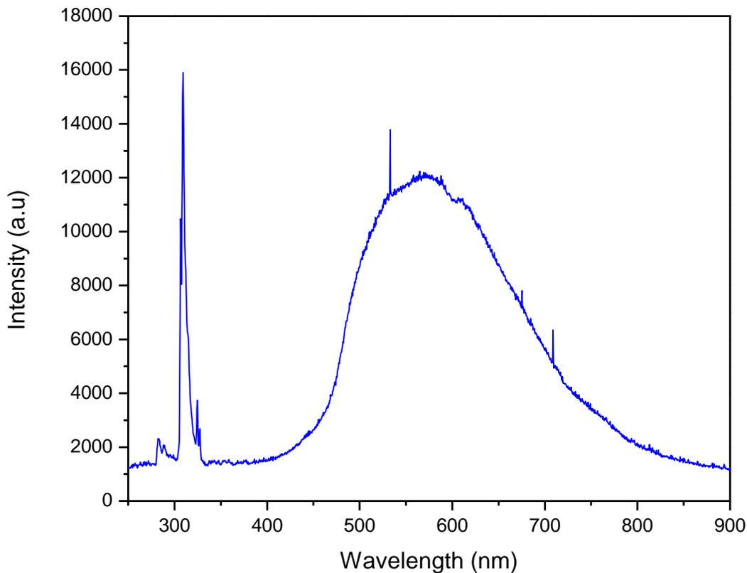
**Figure 9. Optical emission spectrum of air plasma**
