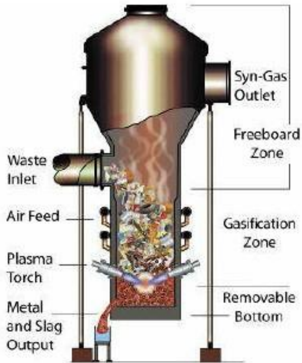
Figure 1: Plasma Chemical Reactor
