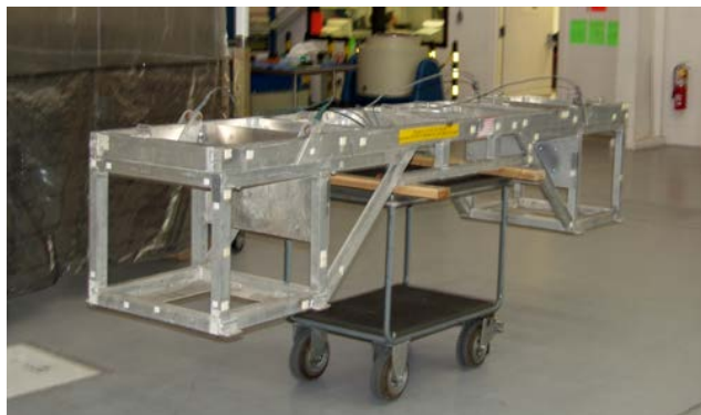
Figure 5. Aluminum unistrut gondola
