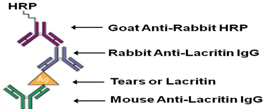
Figure 1. Initial Sandwich ELISA strategy. Capture monoclonal anti-lacritin antibody 1F5-C9-F4 and detector polyclonal anti-N-65 antibodies were respectively generated against lacritin’s N- and C-termini.
