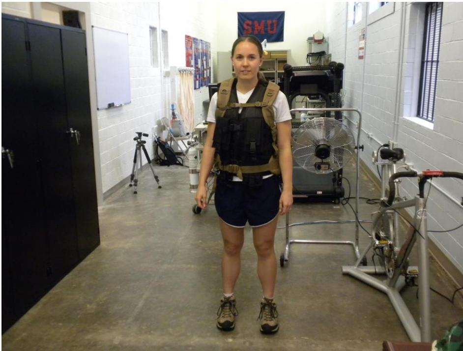
**Figure 2.** The vest and backpack used to add loads to subjects from lateral (A) and front (B) views. Yoga blocks and sealed bags of shot are used to add the condition-specific weight needed for protocol administration for subjects who differ in body mass.
