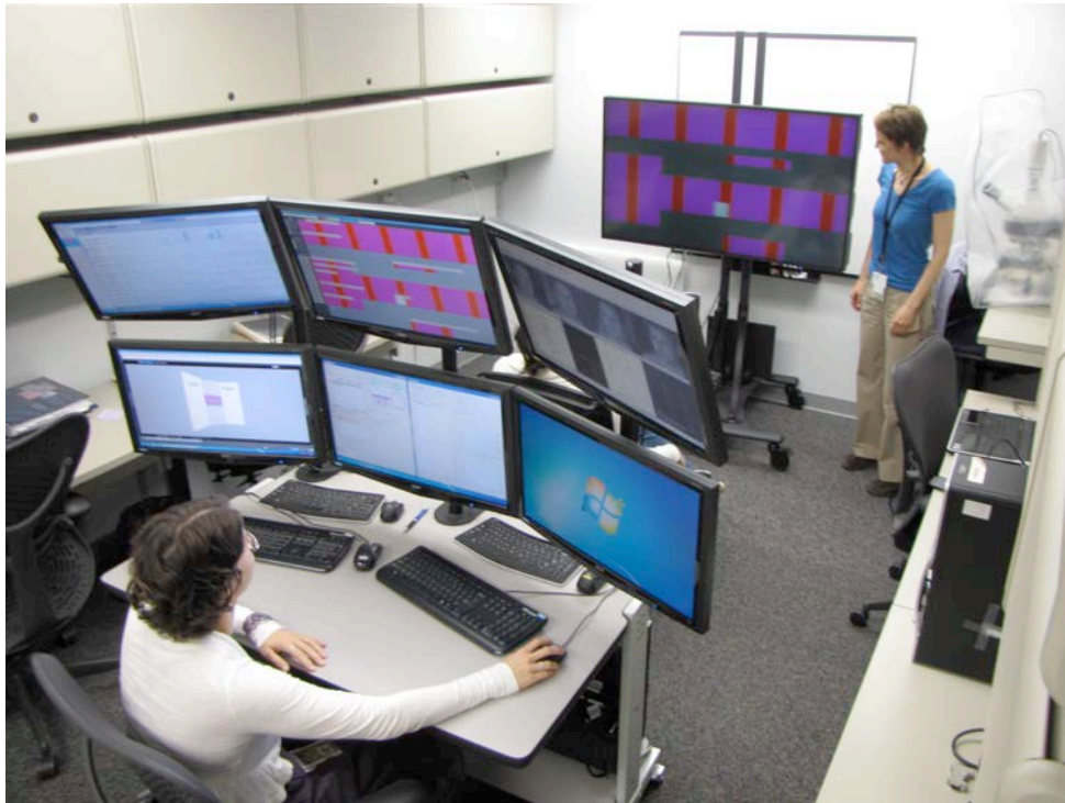
Figure 4: Integrated visual stimulus and analysis platform for recording eye movements, pupil movements and evoked potentials
