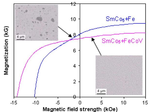
Fig. 3. Demagnetization curves for bulk Sm-Co/ $\alpha$ -Fe magnets pressed at 650  $^{\circ}\text{C}$  after milling for 8 h with starting composition of  $\text{SmCo}_5 + 15\text{ wt}\%$  soft phase (Fe and FeCoV); BSE images of the bulk samples (insets).
