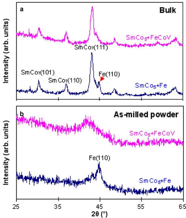
Fig. 4. XRD patterns for (a) bulk samples and (b) as-milled powders with the starting composition of  $\text{SmCo}_5 + 15 \text{ wt}\%$  soft phase (Fe and FeCoV) after milling for 8 h.
