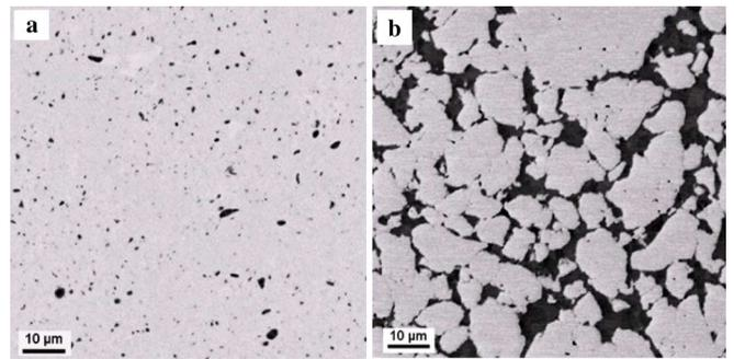
Fig. 6. BSE images for bulk Sm–Co/ $\alpha$ -Fe composite magnets pressed at  $650^\circ\text{C}$ : (a) milled sample of  $\text{SmCo}_5 + 15 \text{ wt}\%$  Fe for milling of 8 h; (b) blended sample of amorphous  $\text{SmCo}_5$  with 15 wt% Fe.
