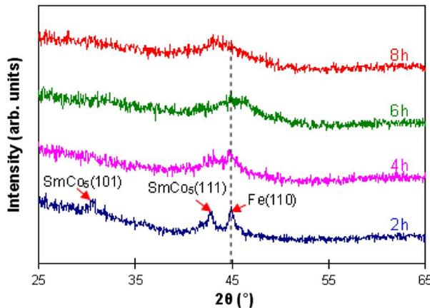
Fig. 5. XRD patterns for as-milled powders with the starting composition of  $\text{SmCo}_5 + 15 \text{ wt}\%$  FeCoV after milling for 2, 4, 6, and 8 h.
