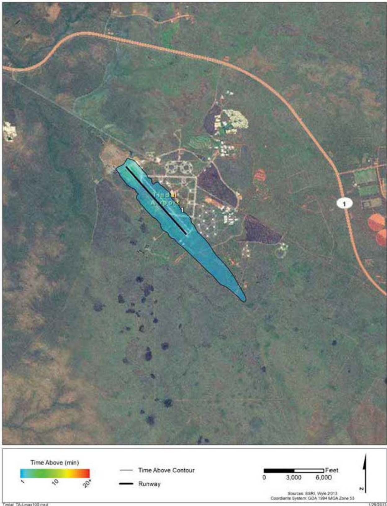
Figure 4-11. TA100 Contours and Gradient for ABD PACAF Aircraft Operations at RAAF Tindal
