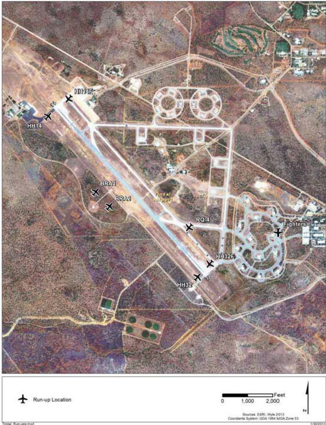
Figure 4-2. Modeled PACAF Aircraft Run-up Locations at RAAF Tindal
