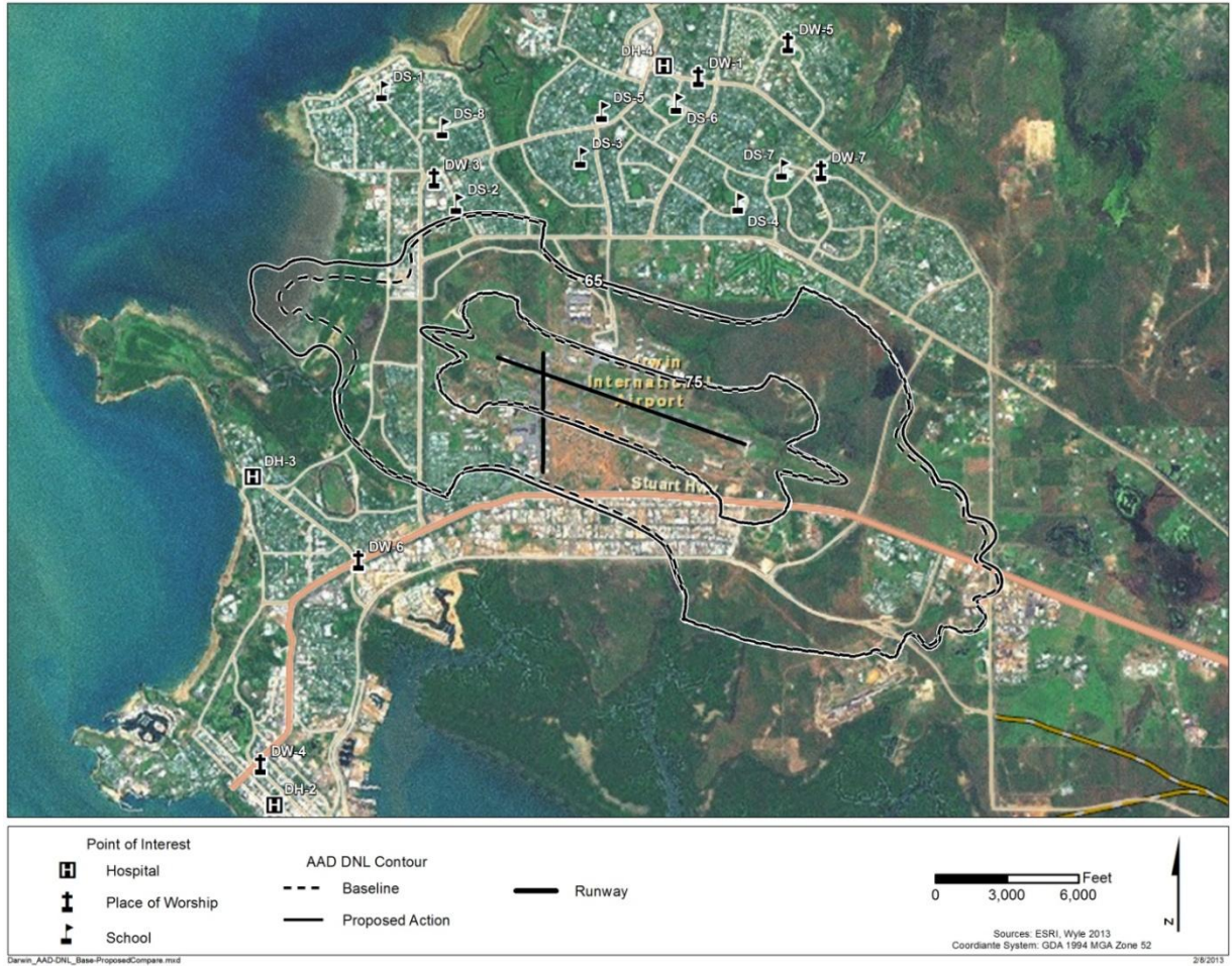
Figure 3-5 Comparison of Baseline and Proposed Action DNL Contours for AAD Aircraft Operations at RAAF Base Darwin PACAF Australia ER
