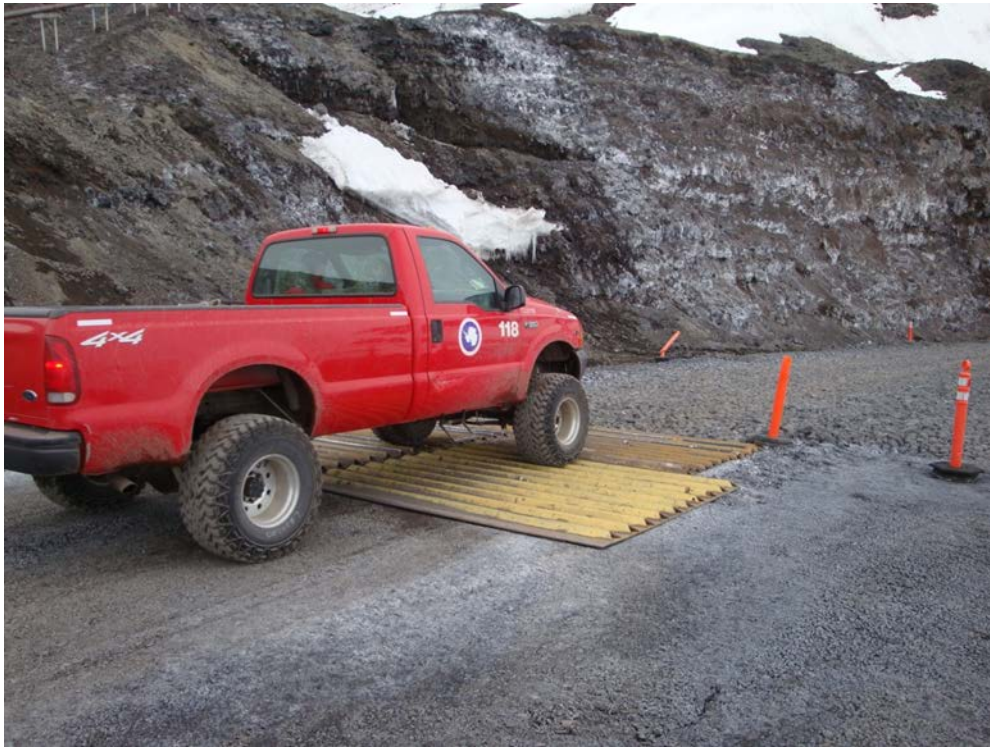
Figure 13. A U.S. Antarctic Program truck crosses the shake plates to clean off debris from the tires and body.
