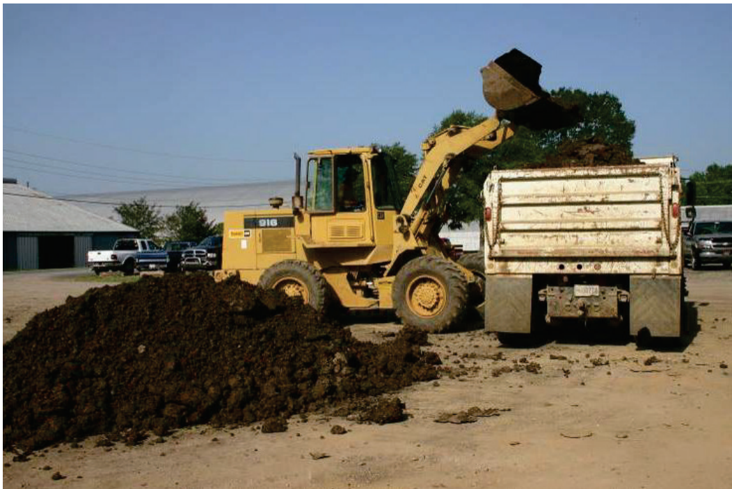
Figure 11. Loading processed CH into haul truck.
