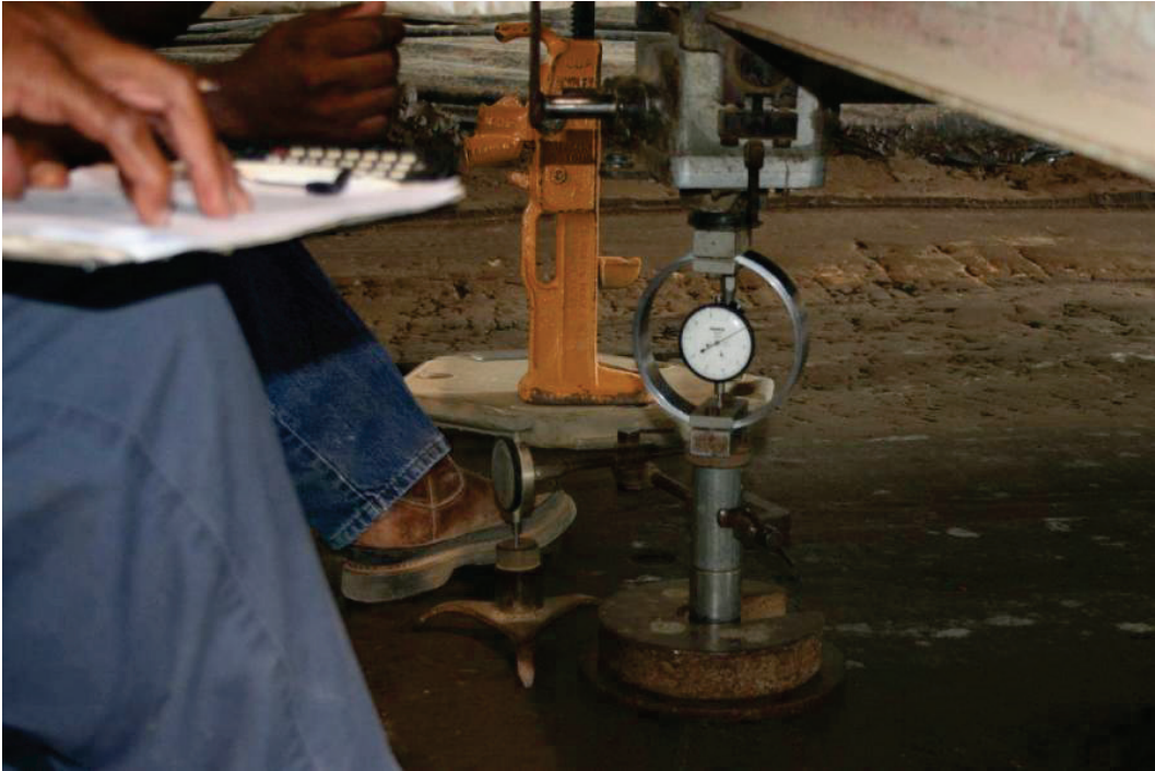
Figure 15. Field CBR test.
