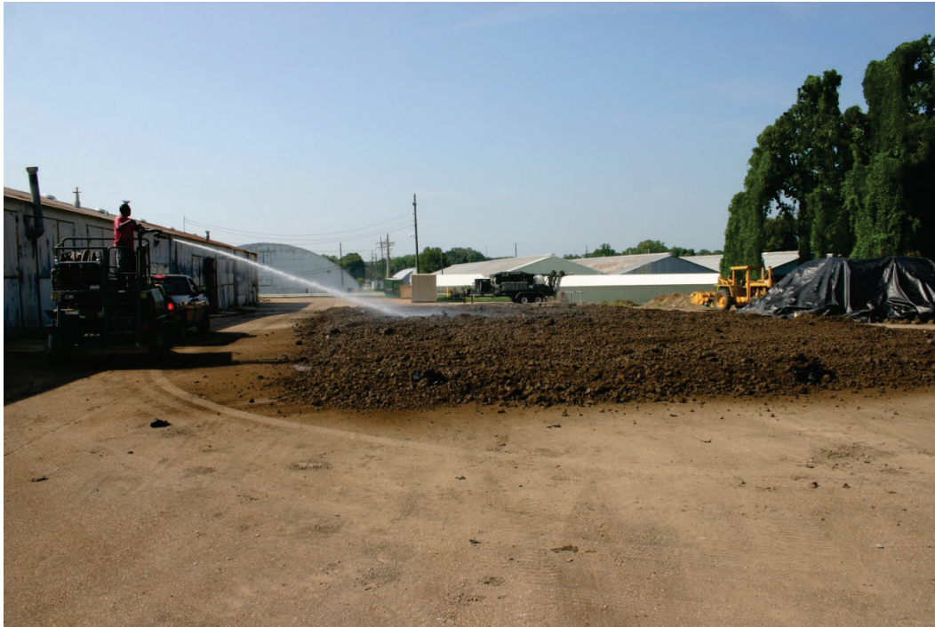
Figure 10. Addition of water to adjust moisture content.
