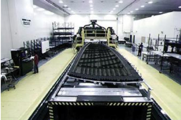
Figure 1-2. NASA and Boeing's advanced stitching machine [Lander 2008].
