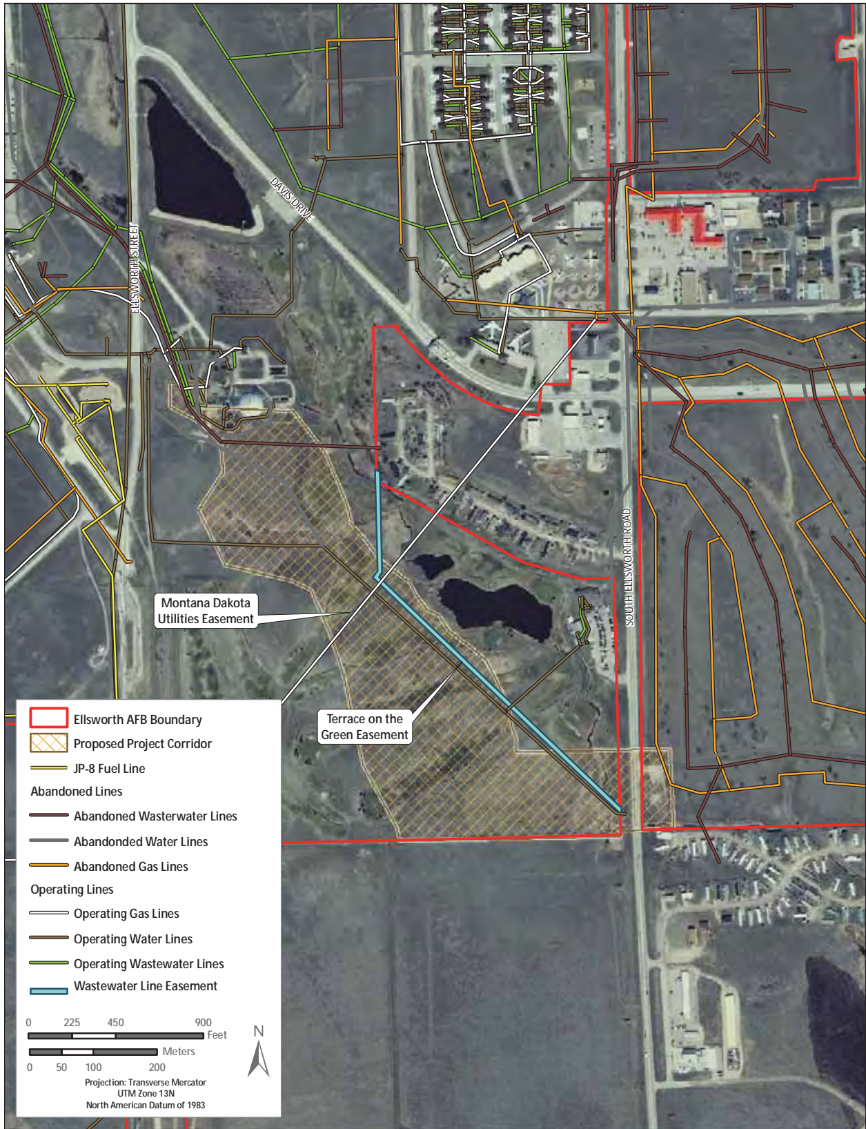
Figure 3-3. Locations of Existing Utility Lines in the Vicinity of the Proposed Project Corridor
