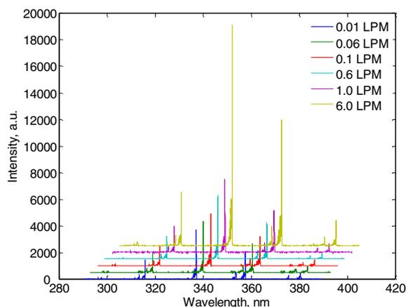
**Figure 7.** Spectra from N<sub>2</sub> DBD discharge between 290 and 390 nm at different gas flow-rates.
