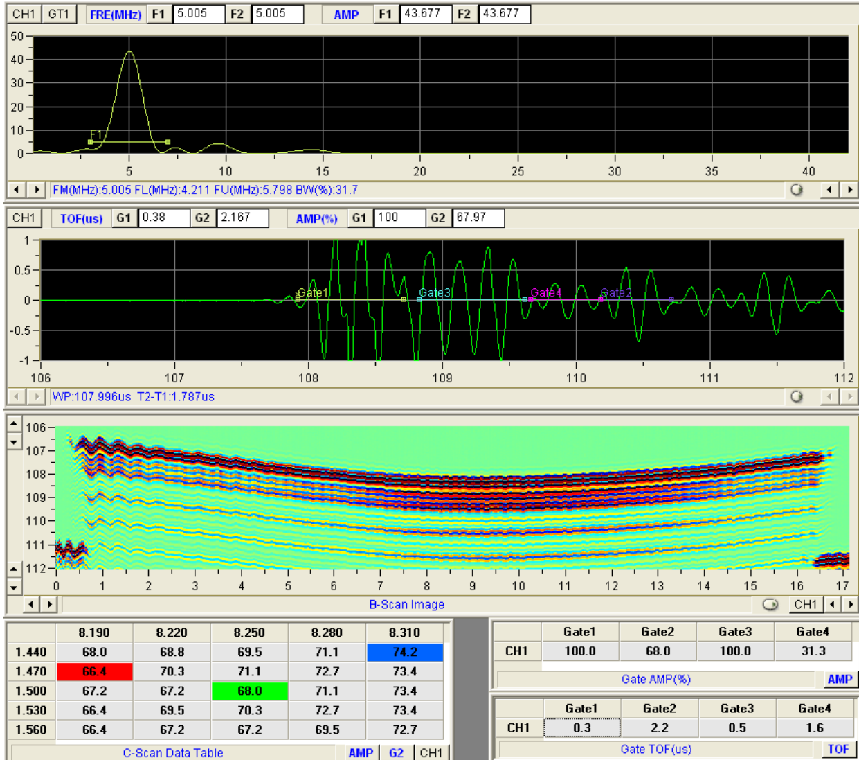
Fig. 4 A-scan, B-scan, and point analysis data from gates 1–4 (top to bottom, respectively)
