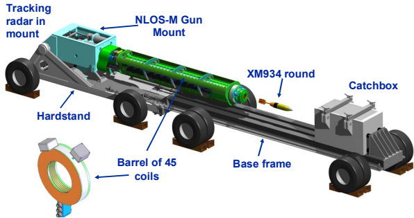
Figure 1. Coilgun mounted in an FCS-type gun mount with catch-box for laboratory tests.
