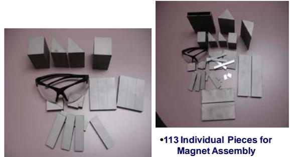
Figure 14 - Magnet configuration, individual parts, and completed final assembly.
