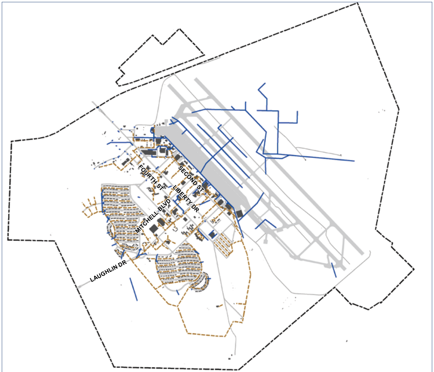
FIGURE 4-14 Sanitary Sewer and Storm Drainage Map
