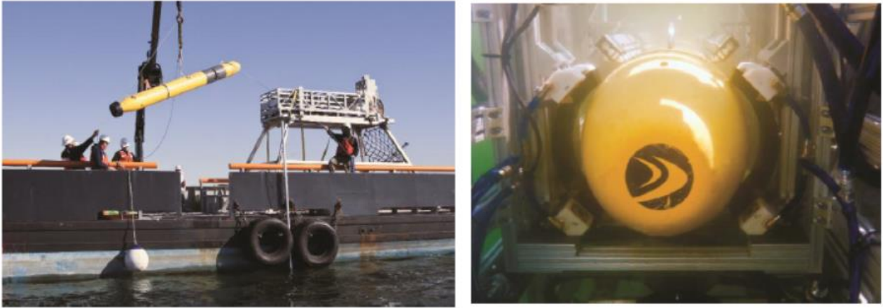
Figure 9: Battelle-developed Docking Station for Bluefin 21 AUV
