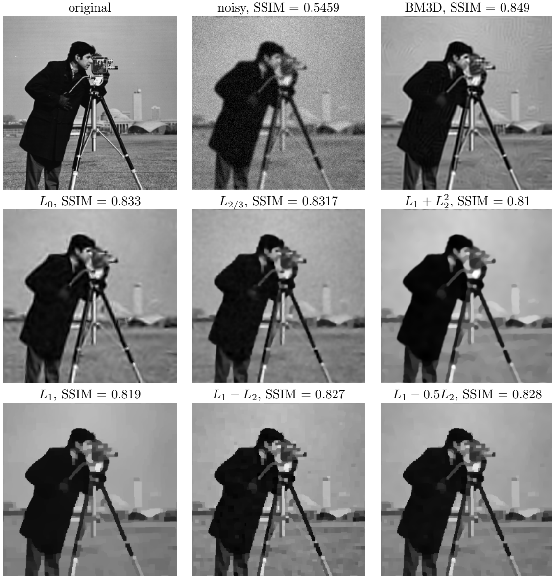
FIG. 3.6. Deblurring results with comparison to L_0 in [31], L_p for p = 2/3 in [21], L_1 + L_2^2 in [2] and the state-of-the-art deblurring method BM3D [11].
