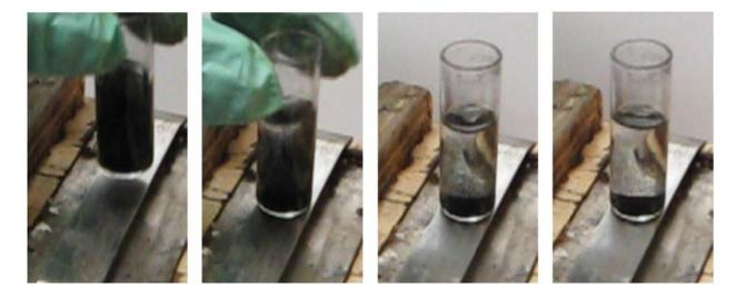
Such work allows for magnetically patternable graphene composites. Simple vacuum-filtered composite films displayed an excellent conductivity of 30 S/m.
