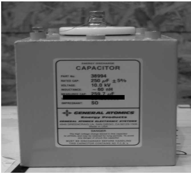
Figure 1. Picture of a single General Atomics capacitor from the newest generation GA-ESI 38994
