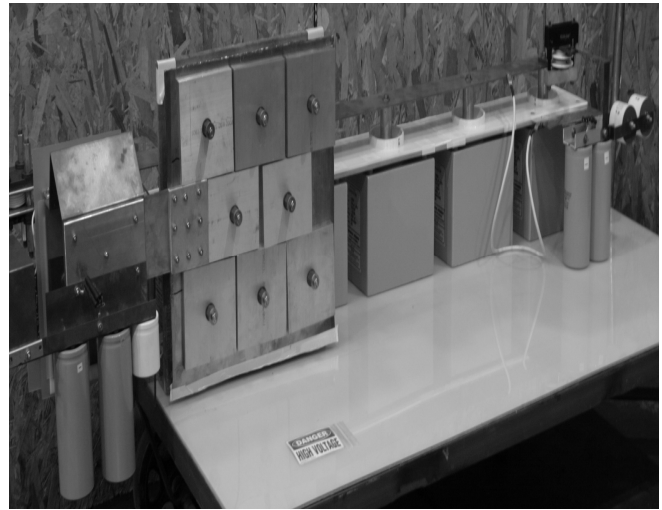
Figure 8. PFN setup involving five capacitors that create a peak current of 200 kA for 100 \mu s.
