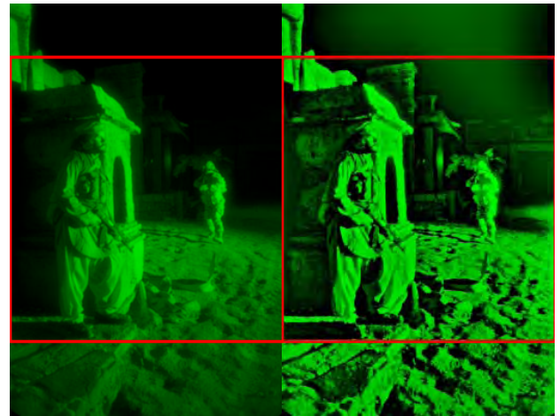
Figure 12: Applying the AR processing to night vision imagery enables the background, hidden in the original (left) to be seen after processing (right)
