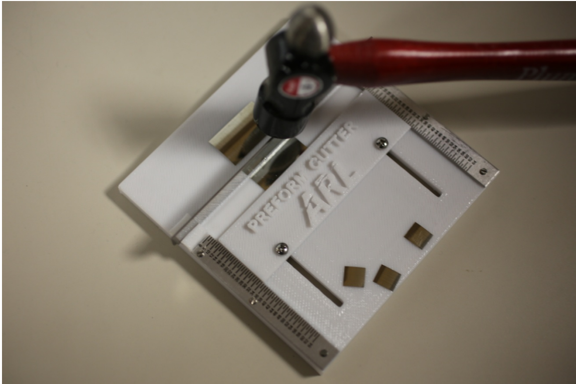
Fig. 5 Solder preform cutter designed and 3D printed at ARL
