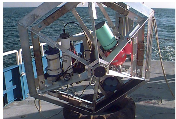
Figure 3. Top: Design and function of bottom-mounted instrument frame. Low-profile pyramidal shape is intended to deflect trawling gear. To enable azimuthally omni-directional acoustic communications, all components other than the acoustic modem transceiver are positioned below the main lobe of the telesonar transducer beam pattern. Bottom: Prototype sensor node frame in upright position recovery.
