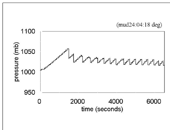
**Figure 3: Pressure record for injection of gas through a fine capillary into a sediment sample from Cow Bay, N.S. at 18 EC**
