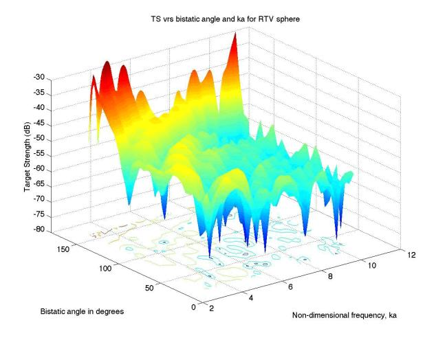
Figure 1: Multi-static scattering from a small RTV sphere. These preliminary data did not extend sufficiently low in frequency to adequately resolve the transition to Rayleigh scattering. That transition, for backscattering, would be near ka = 1.4.
