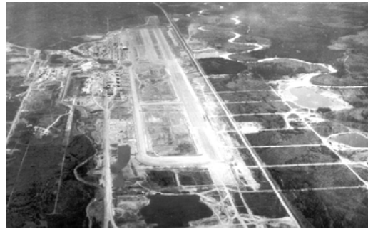
Eielson in 1950. Base development continued through accumulating fill until Eielson AFB's developed area came to resemble an island resting amid wetlands and permafrost within the Tanana River floodplain.
