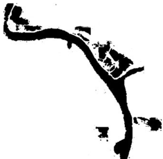
Figure 10. Image in Figure 9 processed for entropy, binarized, opened and closed
