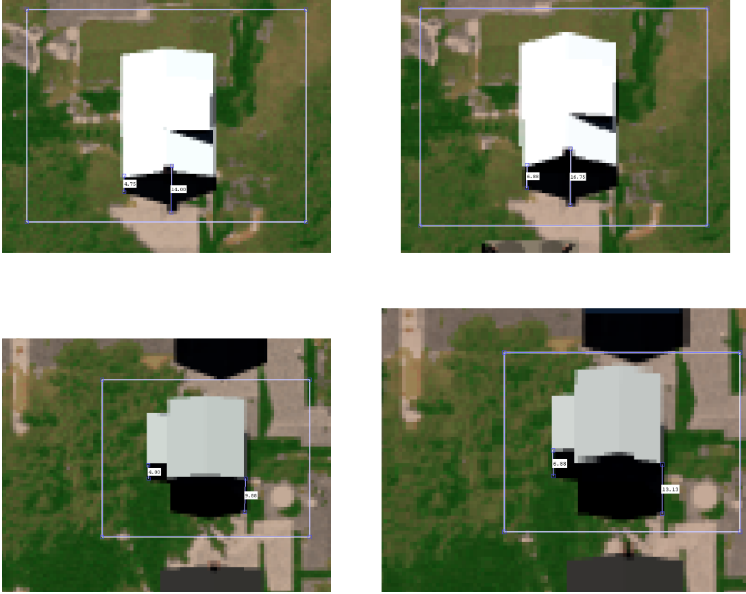
Figure 22. In-scene building edge from the synthetic reference image (collected at a 10^\circ viewing angle) used to manually estimate the parallax direction between images (left images). Synthetic test image (right images) of the same in-scene building but captured from an alternate viewing angle of 20^\circ displaying an increase in visibility of the building side with an appraised parallax shift of 4 pixels in the upward direction ( 90^\circ ). Labels on both image chips are pixel values.
