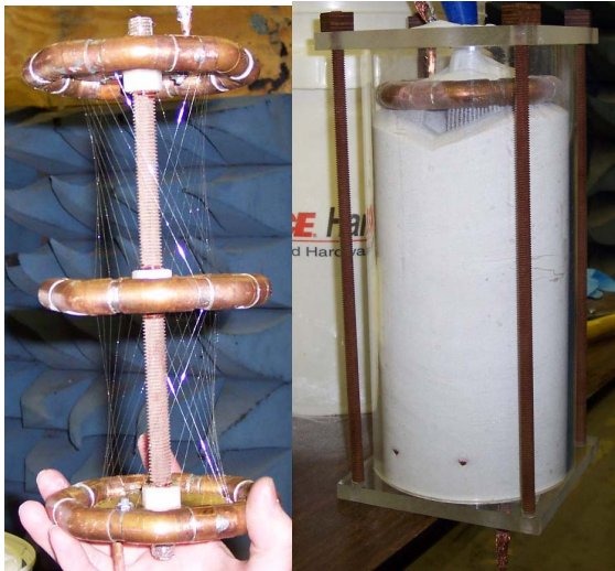
Figure 5. Fuse showing wires and field shapers (left) and being assembled with fine glass beads (right).
