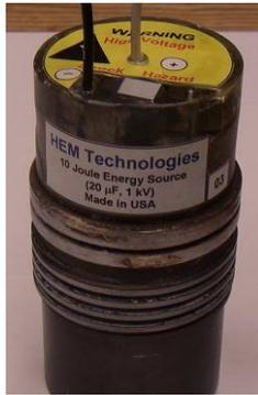
**Figure 2.** Image of 10 J energy source, previously developed by HEM Technologies.
