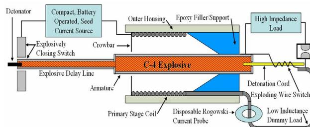
**Figure 1.** Schematic of the complete generator system.
