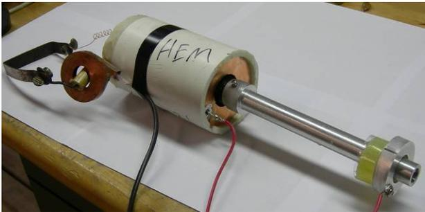
**Figure 3.** Image of complete system including explosively closing switch, delay line, HFCG, fuse wire (without detcord), low inductance load, and current sensor. Seed current generator, connected via the red wires, is omitted.
