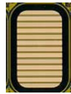
Figure 1. A single Si Super-GTO, cathode side up. Footprint: 2.3 cm long by 1.5 cm wide.
