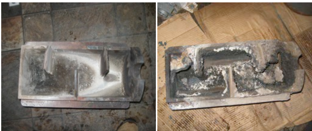
Figure 10. Cast iron tray before installation at McMurdo (left) and after normal usage during the 2011–12 season (right); note the visible caking on the tray on the right.
