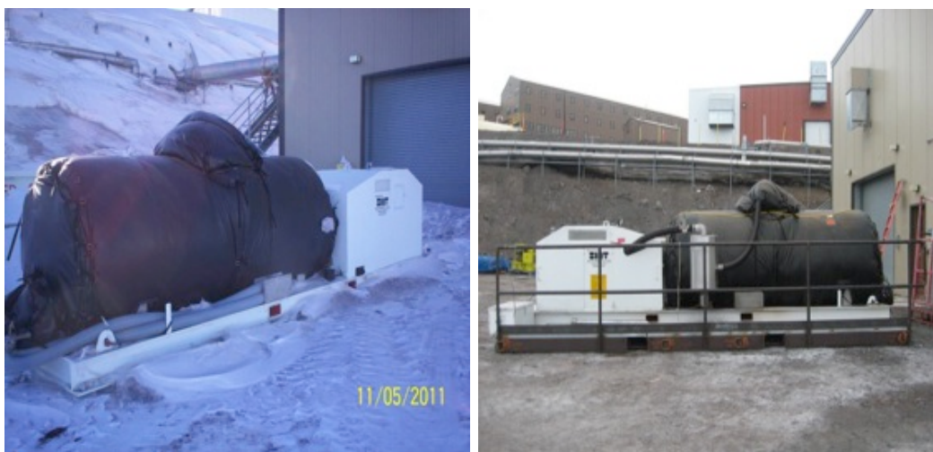
Figure 3. The vacuum tank as delivered (left) and after modification (right).
