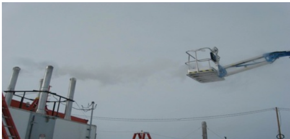
Figure 12. Emissions testing of the incinerator at Pegasus Airfield.
