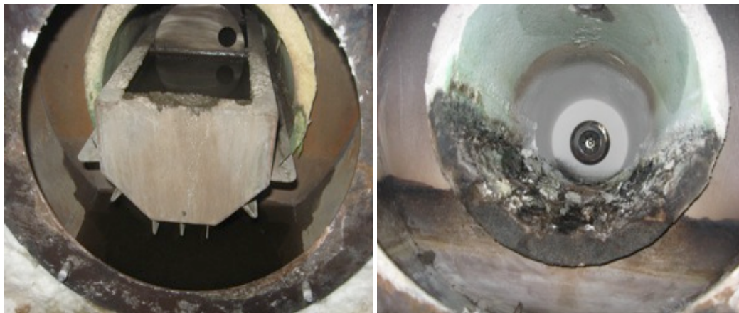
Figure 7. Tray overfilled, causing effluent to spill out of the tray (left) into the exhaust plenum and to leak out of the burner unit onto the floor, saturating the combustion chamber insulation with black water (right).
