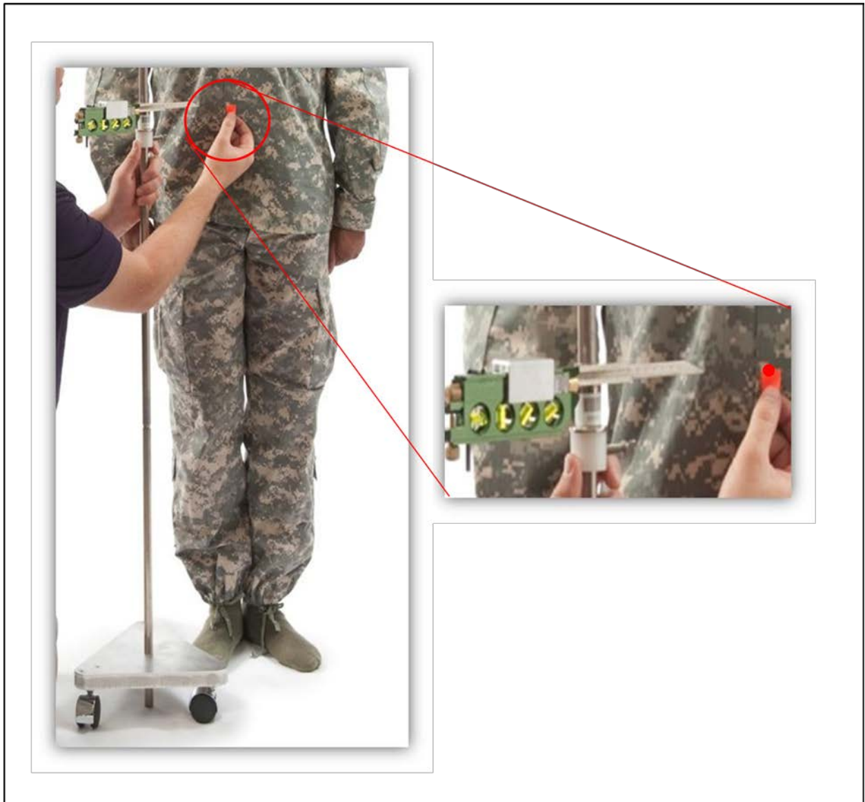
Figure 9: Modified anthropometer used for landmark transfer
