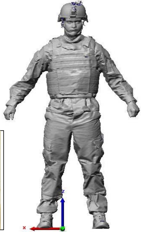
Figure 4: Driver Configuration for obtaining encumbered anthropometric dimensions
