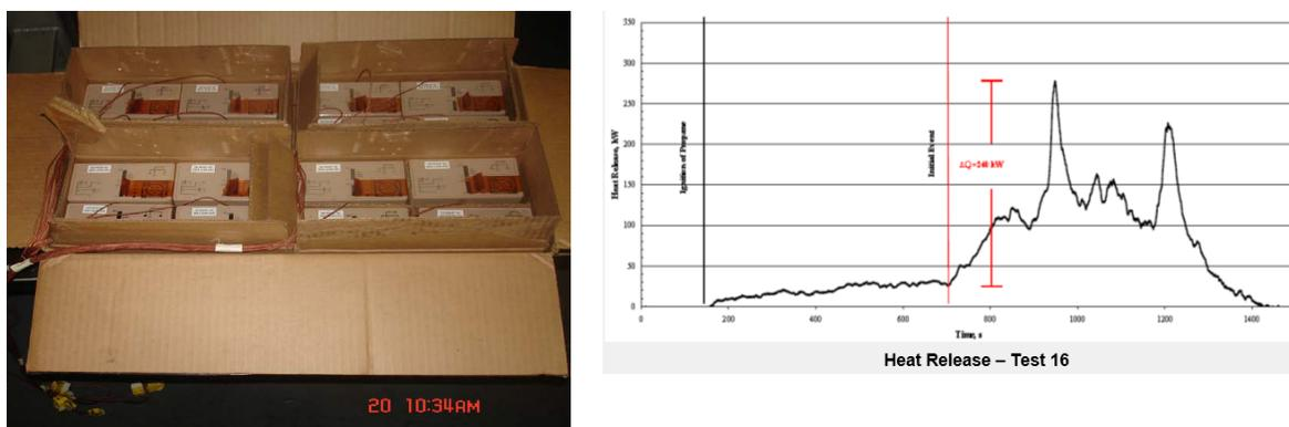
Fig. 10 — Bulk storage test, E type cells
