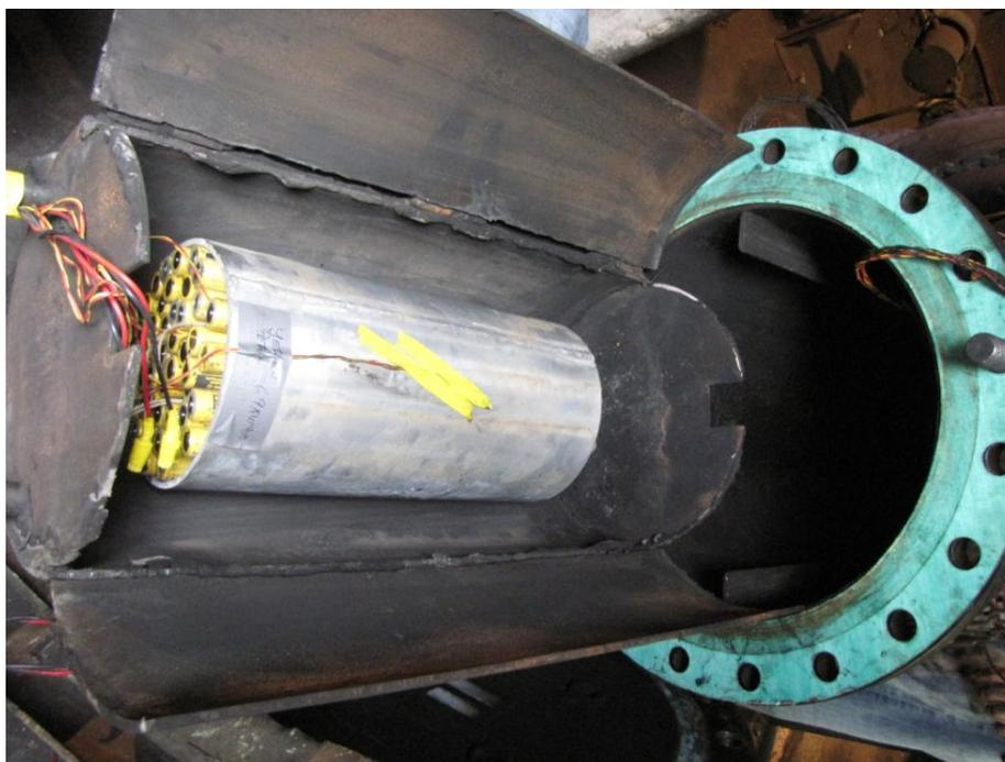
Fig. 14 — Pressurizable containment configuration
