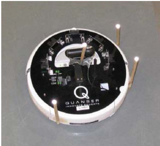
Figure 24: QBot with mounted Infrared Reflectors
