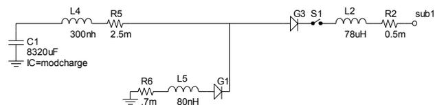
**Figure 1.** Simplified circuit model of single bank module.
