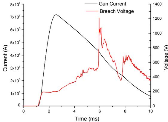
**Figure 5.** Gun current and breech voltage for operation with 10 banks at  $t=0$ , 200 g projectile.
