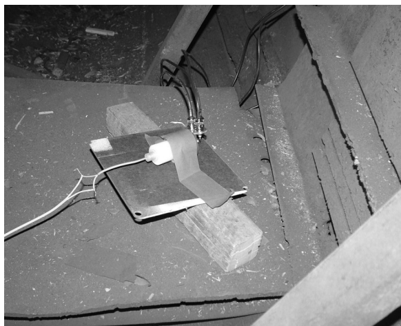
Figure 5. The experimental device containing a KCl sample placed in the detonation tank. Three coaxial 50-Ω signal cables connect three metallic probes embedded in the sample to the external measuring and recording system.
