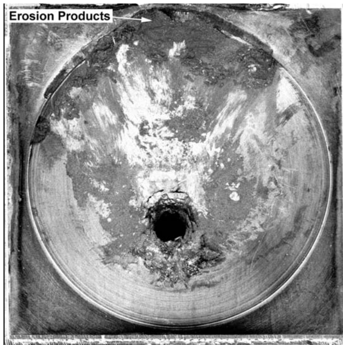
Figure 58. Graphite weak layer cavity recovered from the experiment depicted in figure 55, showing that reduced frontal support and increased ceramic damage did not significantly alter the flow of erosion products.
