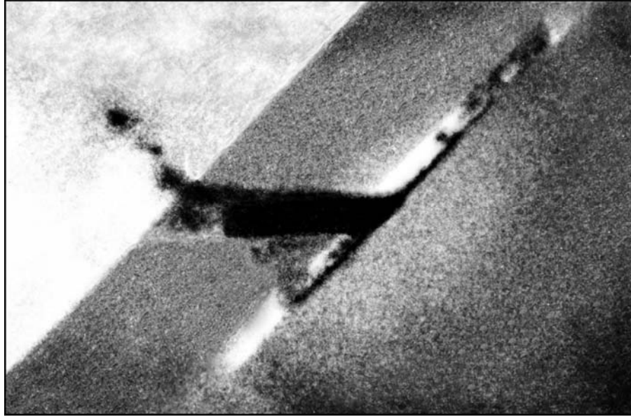
Figure 43. Flash radiograph that shows interface defeat of WHA rod projectile obliquely attacking \text{TiB}_2 ceramic confined by Ti-6Al-4V.
