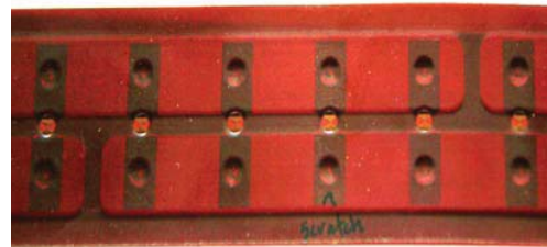
Figure 6. Segment of slapper array showing four bridges in parallel, and one bridge of adjoining series segments.
