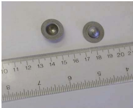
Figure 7. Hemispherical aluminum cups are filled with an HE sensitive to slapper initiation, and one is centered on each slapper. The smallest HE cups that can be used for 18 mm point spacing slappers are 12 mm diameter.
