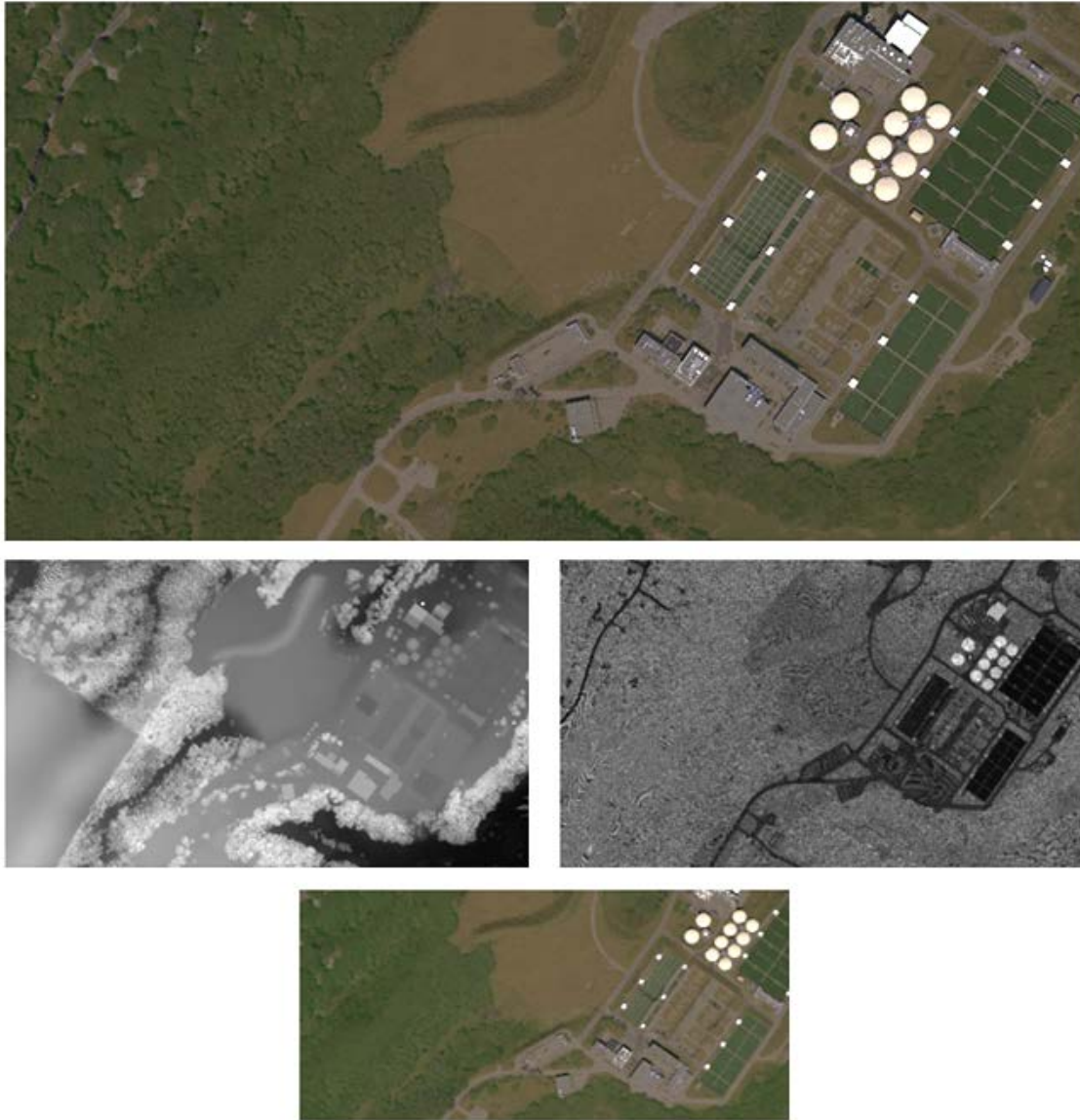
Figure 10. The input DIRSIG generated synthetic imagery. Top: HR imagery, Middle: Lidar elevation and return strength and Bottom: HSI captured over the modeled VanLare Wastewater Treatment Plant near Rochester, NY.
