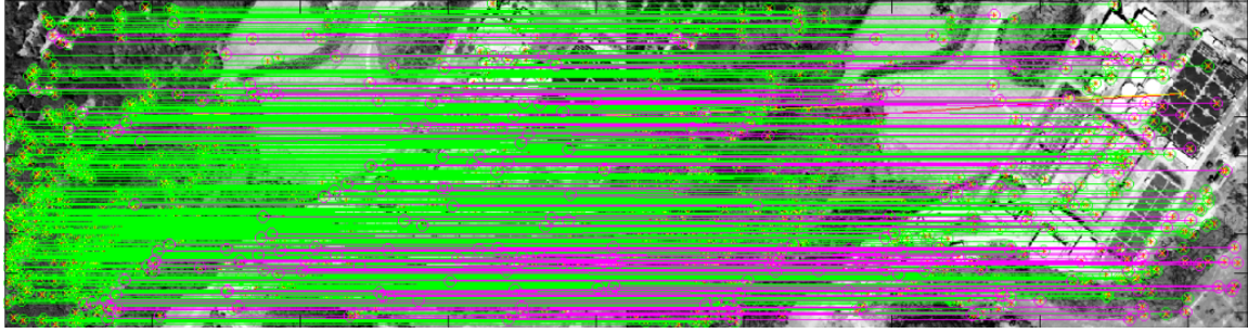
Figure 49. Registration of DIRSIG RGB image and real RGB image of the VanLare scene. The green lines indicate the 692 ‘good’ SIFT matches which survived culling by both RANSAC and RMSDE minimization.
