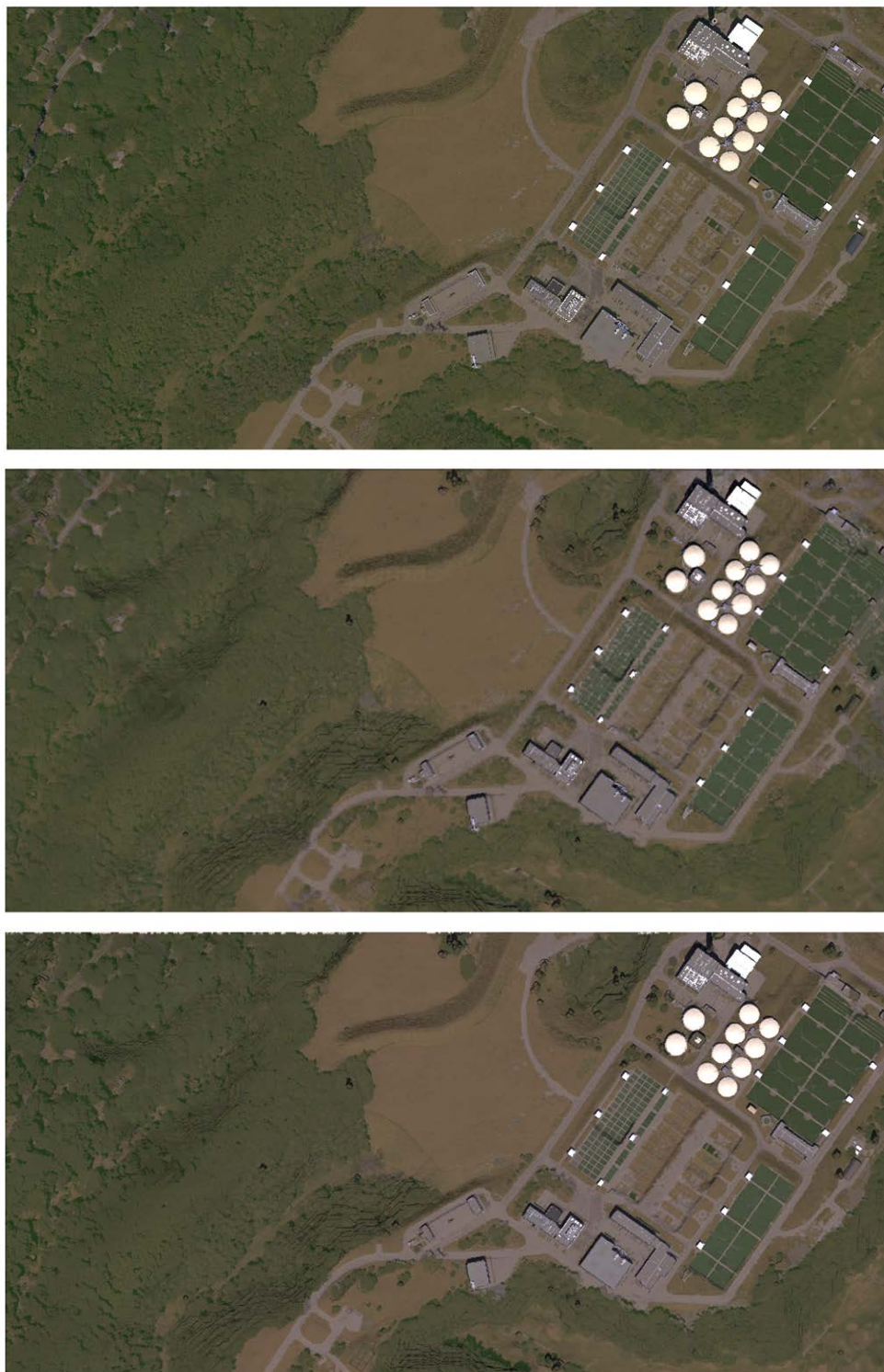
Figure 48. Top: The DIRSIG generated RGB image over the “original” high-fidelity scene at 0.3 meter GSD, Middle: The DIRSIG generated RGB image using the non-fused SEM Approach 1 material map, Bottom: The DIRSIG generated RGB image using the ISODATA fused Approach 3 material map.
