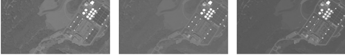
Figure 19. Left to right: The red texture map, green texture map, and blue texture map transformed to the lidar coordinates to be draped over the scene geometry in DIRSIG.
