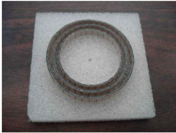
Figure 13: Three layer radome with uniform SRR dimensions in all the layers.
