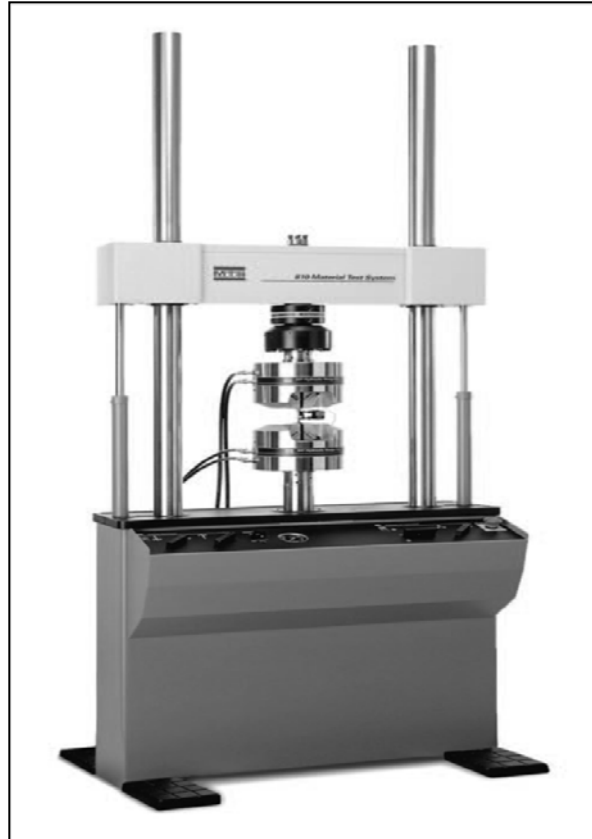
Figure 3.5: The floor-standing 810 mechanical testing system (MTS) [27].
