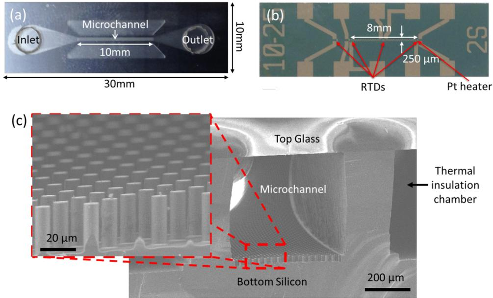
**Figure 2** Images and SEM of fabricated microchannel. (a) Top and (b) bottom view image. (c) SEM of the cross section image of a representative, fabricated microchannel and magnified view of micropillars on the channel bottom surface (inset).
