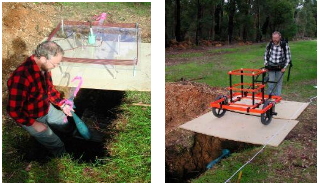
Figure 10 – BEAMOD™ Mk.1 prototype system (left) and EM63 (right) used over the EMIT test pit, Mundaring, Western Australia
