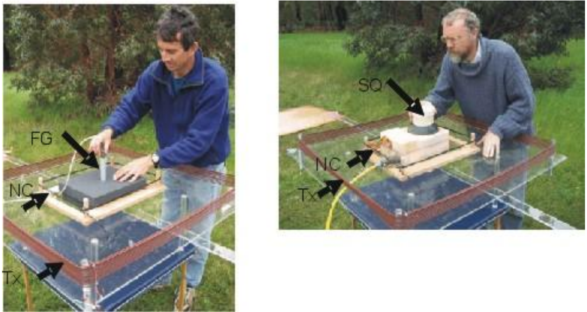
Figure 5 – The BEAMOD™ Mk.1 bench system used for characterization studies on the fluxgate and SQUID sensors.
