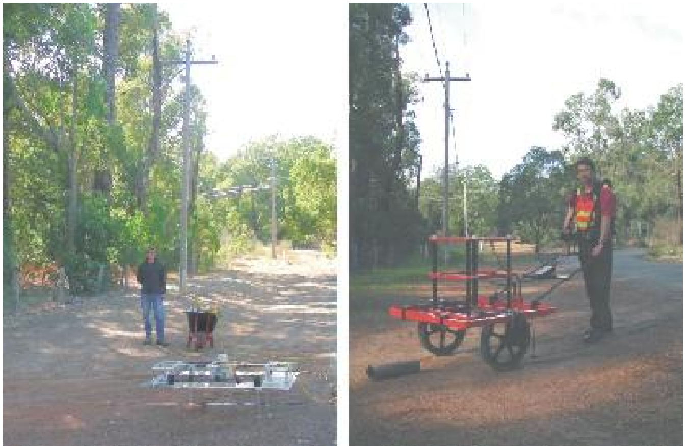
Figure 63 – BEAMOD™ Mk 2 and EM63 instruments in use under high-tension power lines Left: The BEAMOD™ Mk 2 instrument in use under high-tension power lines. Right: The EM63 instrument in use at the same site.
