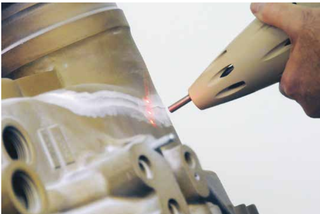
An operator demonstrates repair of an AH-1 helicopter combining gearbox housing using cold spray technology, which enables repairs closer to the field. This will save the Navy $39 million over the next 7 years.
