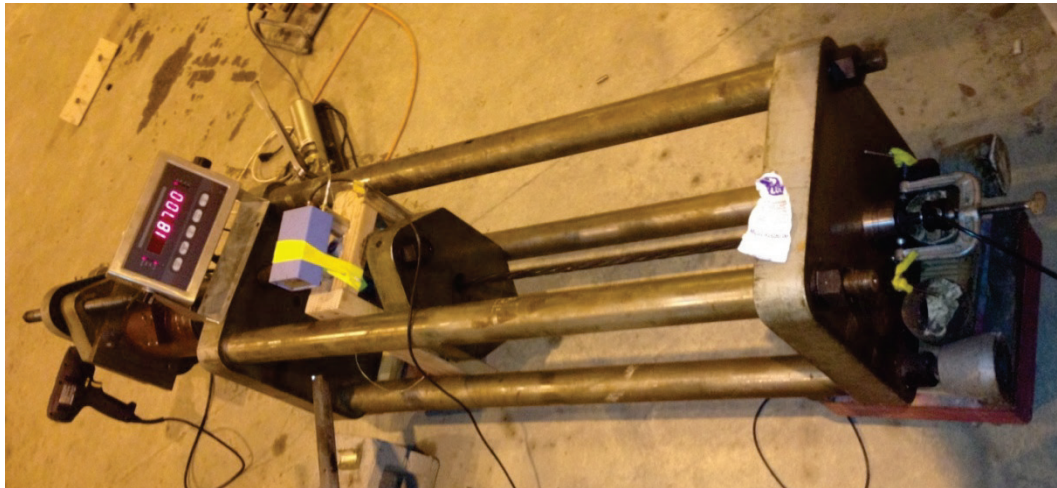
Figure 42. Small hydraulic load frame with fine control of applied tension.
