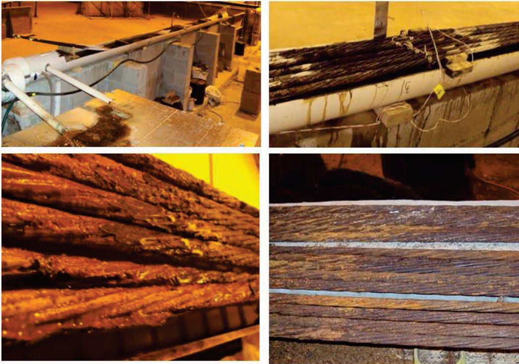
Figure 2. Photographs of corrosion tanks and corroded seven strand wire cables.
