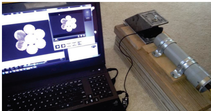
Figure 11. Computer capture with cable installed in imaging frame.
