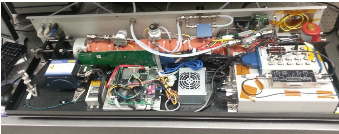
Fig. 3 Photograph of the inside of the CRDS system. The laser head is the blue and white box on the far left of the device. The detector is the red cylinder with a gold top in the upper right-hand corner. The cavity is the orange wrapped cylinder at the top of the unit. Other major components are the laser controller underneath the data acquisition hardware on the bottom right, and the computer in front and in the middle.
